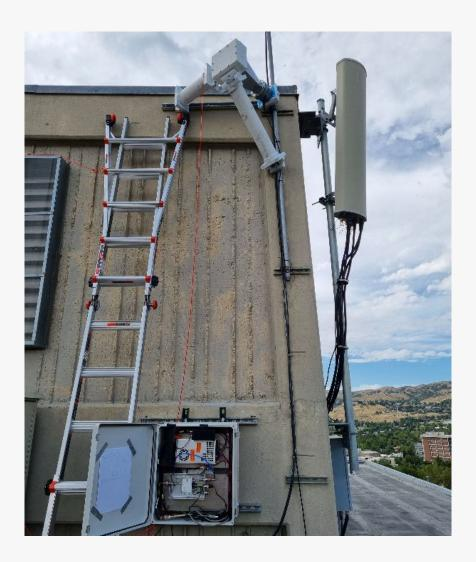
The POWDER team this month supported a long-distance C-band RF measurement study performed by the US Navy. The transmitter for the study was located at the POWDER "Behavioral rooftop" location (as a BYOD deployment), while the receiver was located "off site", approximately 37 km away. The POWDER team provided a horn antenna for the setup (see above) and designed a custom mount to facilitate the deployment of the transmitter.
